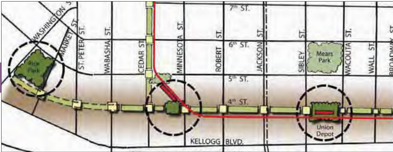
Figure 2.25 Opportunities to improve the public realm along 4th and Cedar streets in conjunction with LRT are limited due to the narrow right-of-way within which the train and associated hardware must fit. In particular, the frequency of vaults and areaways under sidewalks, and the proximity of LRT to the curb significantly limit possible locations for street trees. In response, public realm plantings will follow a pattern of urban gardens and urban forests along 4th and Cedar. Urban gardens (including large potted plants, hanging baskets and window boxes) will be planted along the street faces between stations. Urban forests (i.e. trees) will be concentrated at stations.
